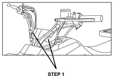
Insert the gear indicator on the handlebars.
